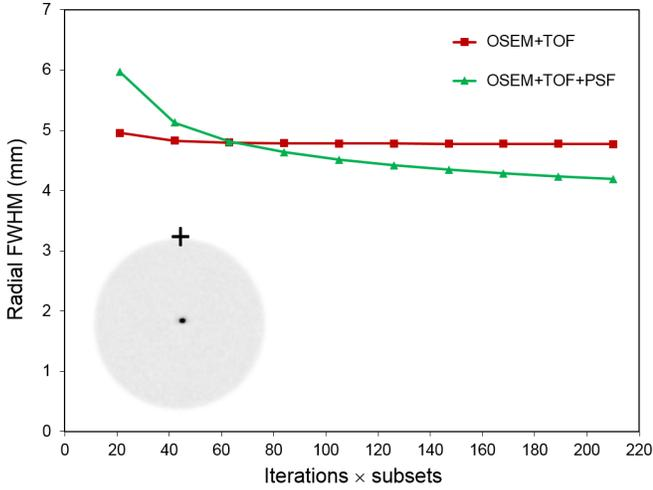
Fig. 2. Spatial resolution (radial component) measured using a point source in a radioactive background. The inset image shows the experimental arrangement with the center of the field-of-view indicated by a cross. Data are shown for OSEM+TOF and also OSEM+TOF+PSF.
