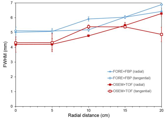
Fig. 3. Spatial resolution derived from in-air point source measurements at various distances from the center of the field-of-view. Results with FORE+FBP and OSEM+TOF (2 iterations) are shown for both radial and tangential directions.
