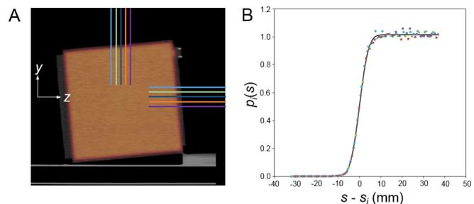
Fig. 1. (A) A uniform cylinder positioned at an oblique angle shown in sagittal orientation. (B) Line profiles across the phantom edge in the  $y$ -direction allow measurement of the radial component of spatial resolution. The oblique angle allows for very fine sampling of the edge spread function,  $p_r(s)$ , when multiple slices are combined.
