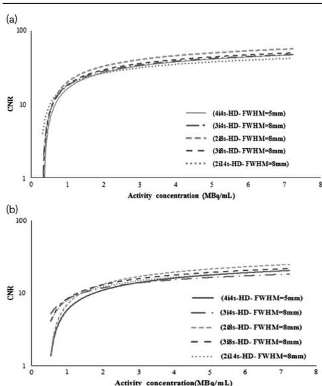
CNR versus true activity concentration in a syringe with (a) 30.5 mm of diameter and (b) 9.15 mm of diameter for different optimized reconstruction parameters. CNR, contrast-to-noise ratio; FWHM, full-width at half-maximum.
