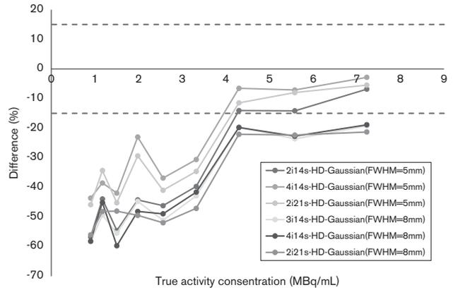
Differences in the measured activity concentration in all syringes with respect to the true activity concentration for various reconstruction parameters over nine imaging time-points. FWHM, full-width at half-maximum.
