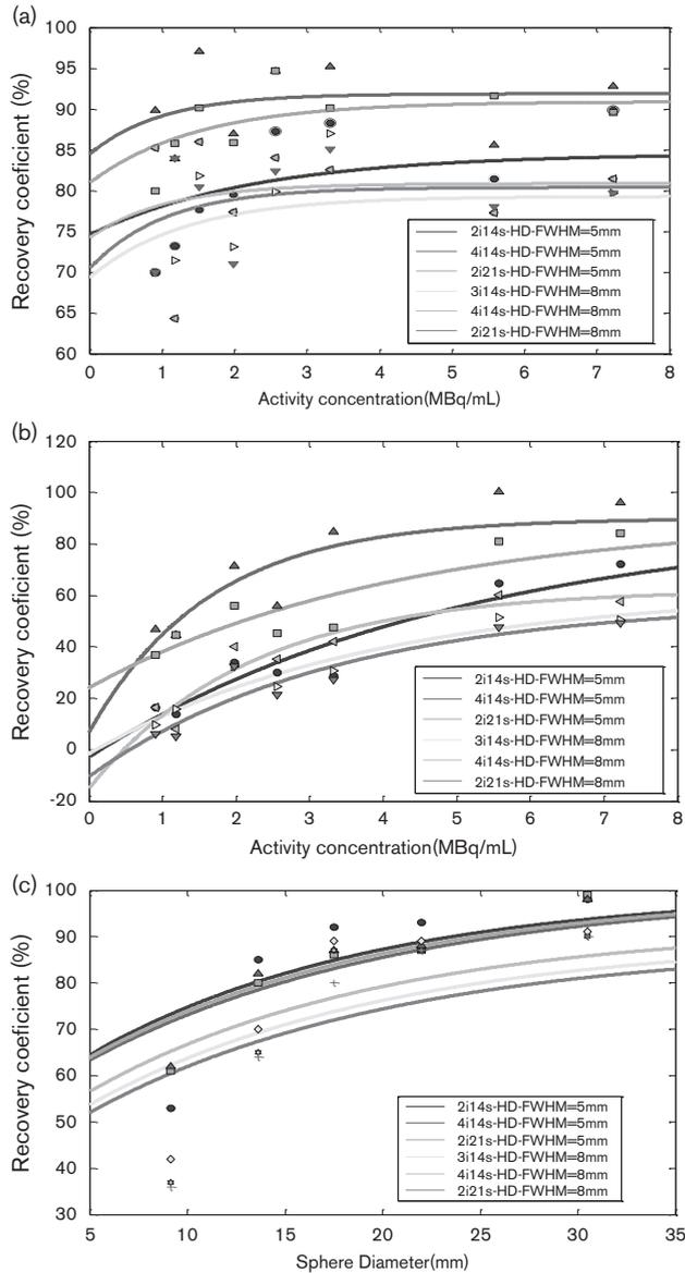
Recovery coefficient for (a) 30.5-mm diameter syringe, (b) 9.15-mm diameter syringe at different activity concentrations, and (c) in hot syringes of different diameters on the first day of imaging considering the optimized reconstruction parameters for quantification accuracy. FWHM, full-width at half-maximum.
