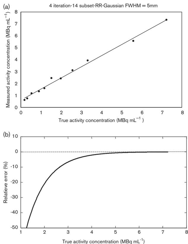
True activity concentrations versus measured activity concentrations (a) and the associated relative errors (b). FWHM, full-width at half-maximum.
