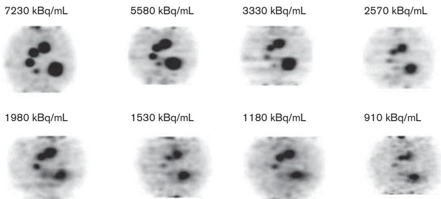
Transverse PET/CT slice of the Jaszczak phantom, crossing all five hot syringes (internal diameters of 30.5, 22, 17.5, 13.65, and 9.15 mm) for eight imaging time-points using the optimized reconstruction parameters.
