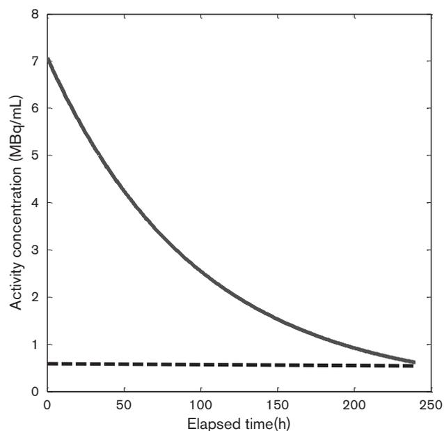
The average of the measured activity concentrations in hot syringes using PET/CT, without background subtraction versus time.
