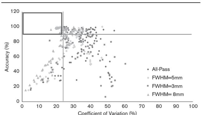
Accuracy and coefficient of variation (CoV) for all the reconstructed activity concentrations. The box indicates the suggested reconstruction parameters. FWHM, full-width at half-maximum.
