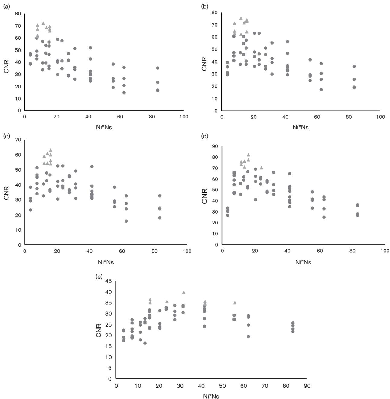
The CNR values for various reconstruction parameters for (a) 30.5-mm, (b) 22-mm, (c) 17.5-mm, (d) 13.6-mm, and (e) 9.15-mm diameter syringes (triangular points are the top CNR values corresponding to the highest detectability). CNR, contrast-to-noise ratio;  $N_i$ , number of iterations;  $N_s$ , number of subsets.
