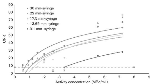
Plots, and lines of best fit, for CNR in hot syringes of various diameters versus activity concentration for the optimized reconstruction parameters. CNR, contrast-to-noise ratio.
