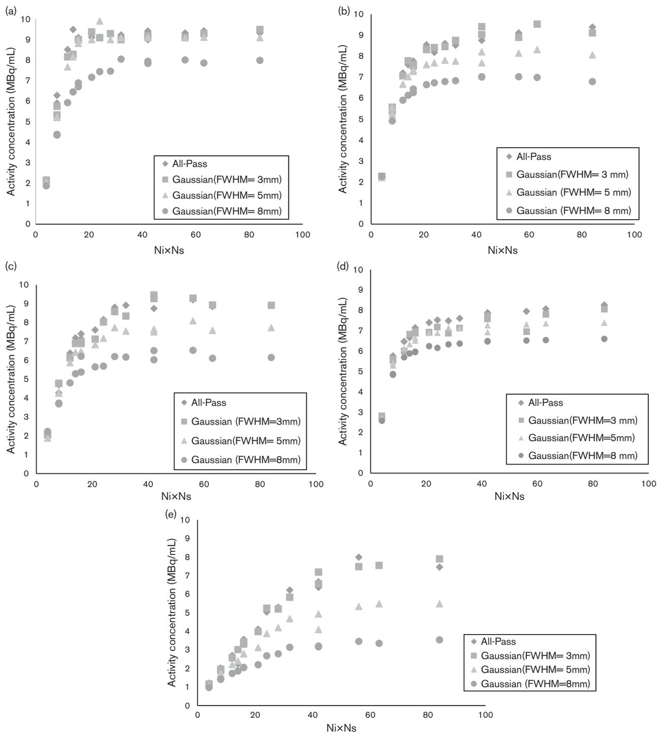
Measured activity concentration versus various number of subiterations for syringes with a diameter of 30.5 mm (a), 22 mm (b), 17.5 mm (c), 13.65 mm (d), and 9.15 mm (e). FWHM, full-width at half-maximum;  $N_i$ , number of iterations;  $N_s$ , number of subsets.
