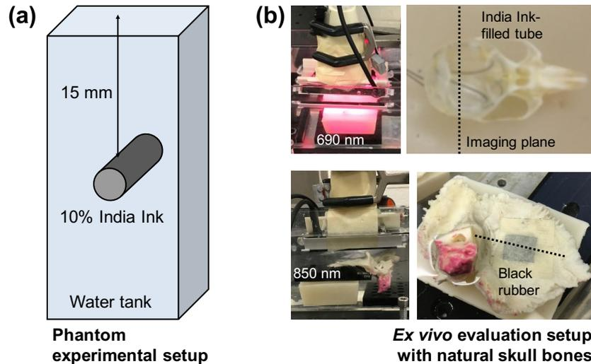
**Figure 2** *Ex vivo* transcranial photoacoustic imaging setup using near-infrared pulsed LED illumination system: (a) phantom experimental setup at 850 nm, (b) mice skull imaging at 690 nm, human temporal bone imaging at 850 nm, respectively.
