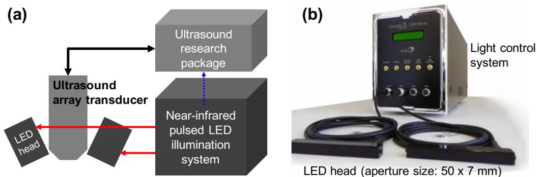
**Figure 1** Preliminary experimental setup: (a) system configuration, (b) near-infrared pulsed LED illumination system
