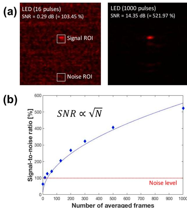
**Figure 3** Phantom experimental results; (a) photoacoustic images at different number of frames for temporal averaging (i.e., 16 vs. 1,000), (b) signal-to-noise ratio versus number of averaged frames
