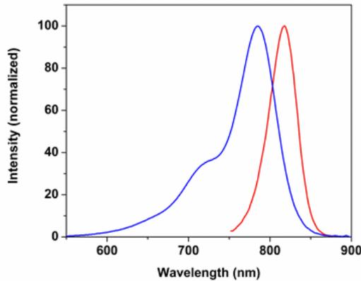
Fig. 2: ICG absorption (blue) and emission (red) spectrum [4].
