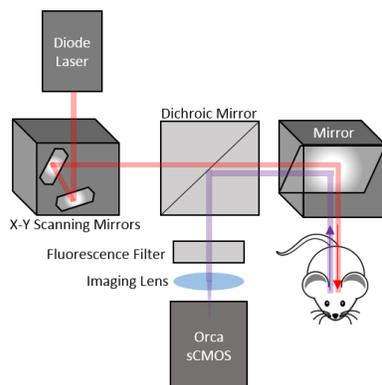
Fig. 1: Fluorescence imaging system
