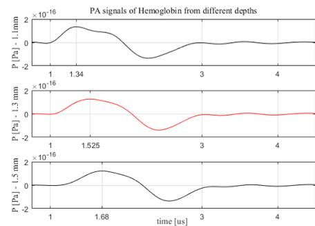
Figure 10: PA signals of Hemoglobin from depths of 1.1 mm, 1.3 mm and 1.5 mm under the surface of mouse head. The shortest depth has a faster pressure amplitude maximum.
