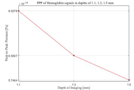
Figure 11: decreasing of PPP due to increasing the PAM depth.
