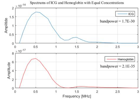
Figure 9: Power Spectrums of ICG (blue) and Hemoglobin (red) with equal concentrations. Their bandpowers are indicated too.
