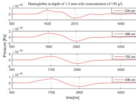
Figure 3: PA signals of Hemoglobin from depths of 234, 468, 702 and 936 μm. The sensing time increases with increasing size.
