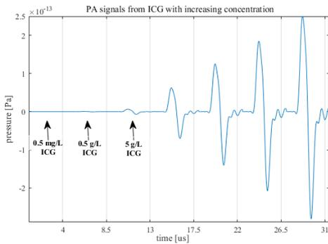
Figure 6: time-domain PA signals from different concentrations of ICG.
