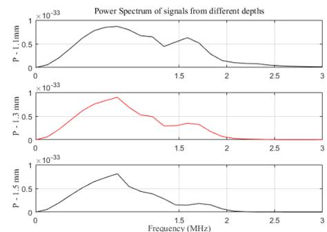
Figure 12: Power Spectrums of PA signals from depths of 1.1mm, 1.3mm and 1.5mm under the surface of mouse head.
