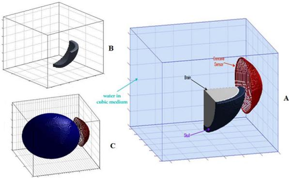
Figure 1: Mouse Brain phantom and focused sensor used in simulation.
