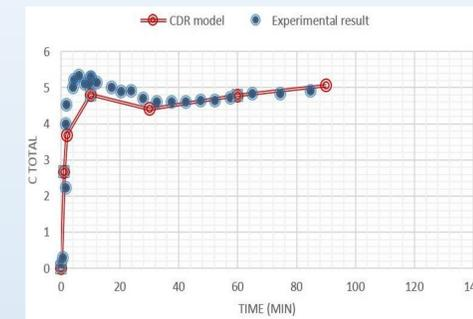
Fig. 3: Comparison of average concentration of FMISO ( $C_{total}$ ) in tumor region with experimental data
