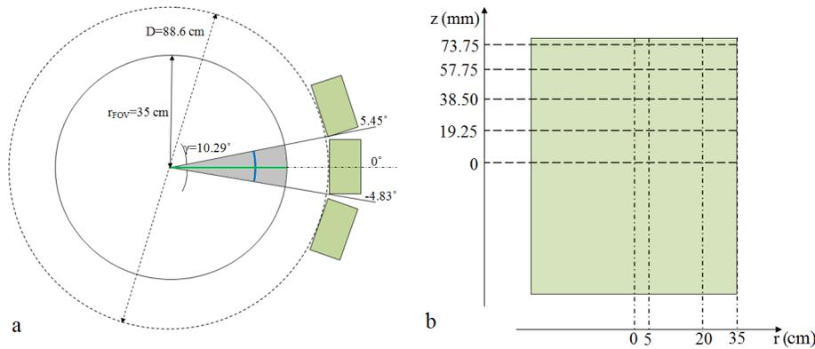
Fig. 3. (a) Cross section of the DRX gantry in which the green line and the blue arc are the locus of points assessed in radial direction and angular direction, respectively; (b) Top view of the DRX gantry in which the locus of investigated points in axial direction are shown. The dimensions in Z-direction are exaggerated.
