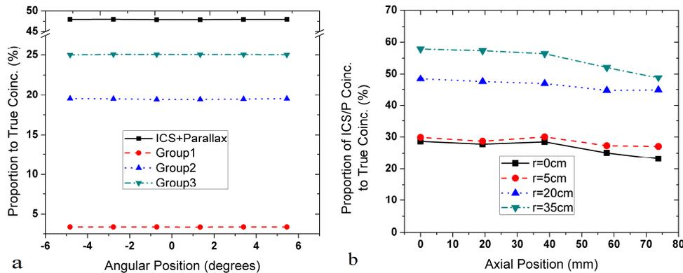
Fig. 4. The proportion of ICS-P coincidences to true coincidences in DRX (a) along the angular direction in one angular period at radius of 20 cm; and (b) along the axial direction at four different radial positions.
