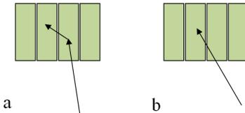
Fig. 1. An example of a photon experiencing (a) ICS and (b) penetration in a typical detector block.
