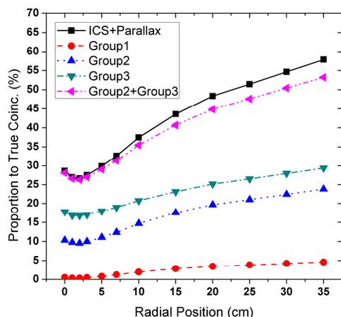
Fig. 5. The proportion of ICS-P and the triple groups coincidences to true coincidences along radial direction in DRX.
