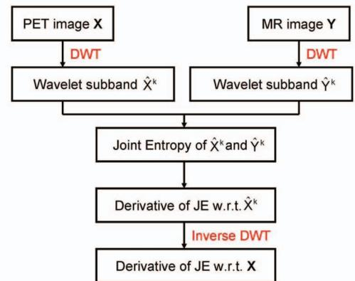
Figure 3: Diagram for calculating derivative of subband joint entropy with respect to the full PET image voxel intensities, DWT: discrete wavelet transform.
