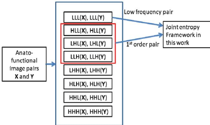
Figure 2: Joint entropy calculation scheme of wavelet subbands.
