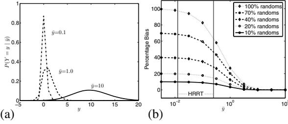
Fig. 1. (a) The probability  $P(Y = y | \bar{y})$  as function of  $y$  (random fraction is 20%). (b) PB due to zero-thresholding.
