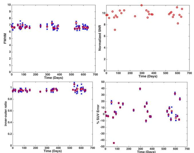
**Figure 1:** Site A - Plots of (*top left*) FWHM, (*top right*) SNR, (*bottom left*) uniformity, and (*bottom right*) SUV accuracy, over time. For a given date, blue x's indicate the results for each of the 4x5min frames, while the red circle indicates the results for the overall summed image.
