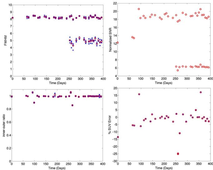
**Figure 2:** Same as Fig. 1 but for site B. Starting ~250 days after first scan, a new reconstruction protocol with reduced smoothing was added. This considerably improved effective resolution, but degraded SNR.
