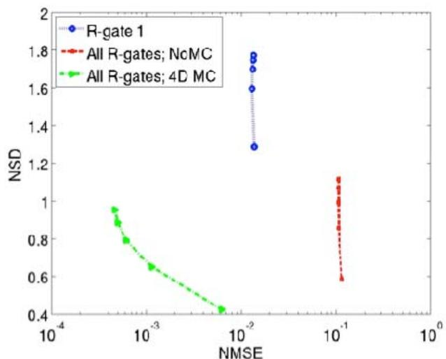
**Fig. 3:** Noise (NSD) vs. bias (NMSE) plots for images of cardiac gate 1 reconstructed with data from (a) only first resp. gate, and all resp. gates with (b) no MC and (c) proposed 4D MC technique.
