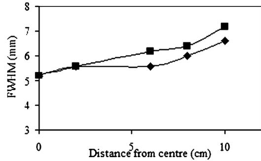
Fig. 3. Axial (squares) and radial (diamonds) resolution measured for the ECAT 953B.
