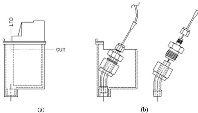
Fig. 1. (a) Side view—cut lines on printer ink cartridge. (b) Side View—section and assembly of modified ink cartridge.
