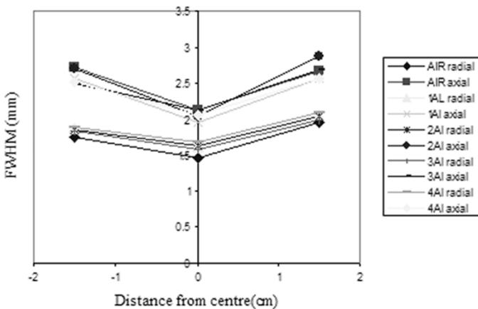
Fig. 7. Axial (top set of curves) and radial (bottom set of curves) PSF FWHM measured for the microPET.
