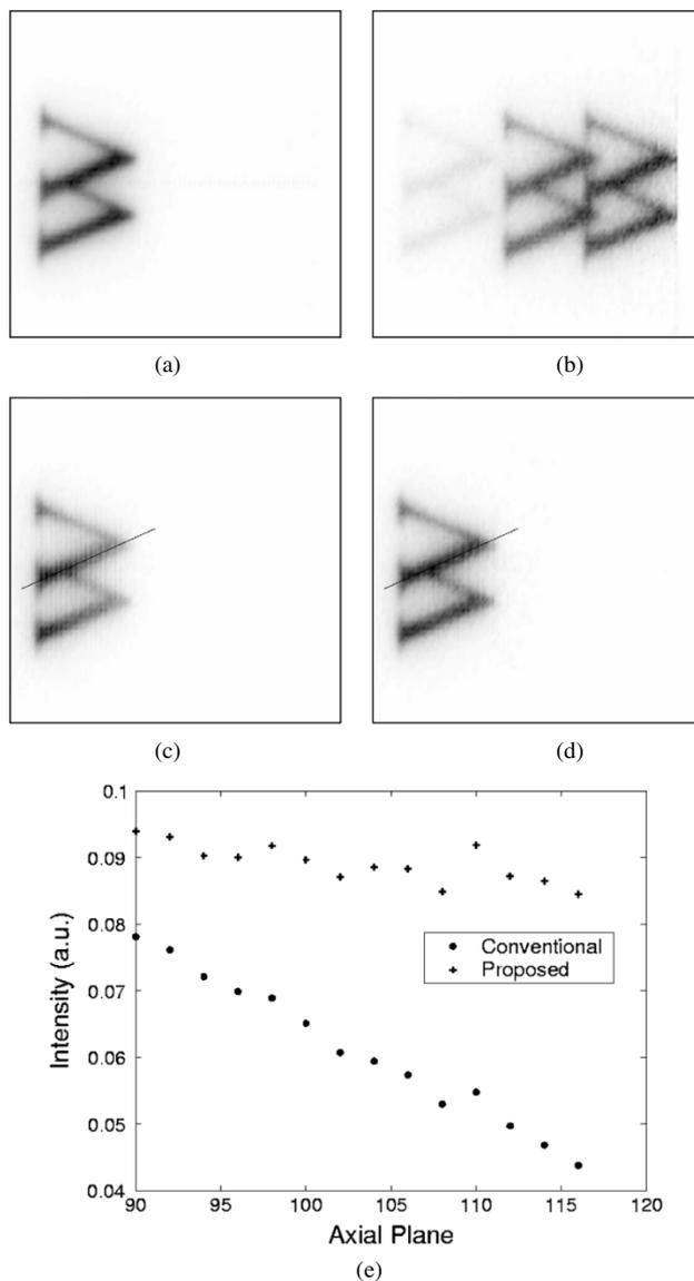
Fig. 5. Images reconstructed for a radioactive printed “W”-sign (coronal view) when (a) no motion is introduced; and with motion (three axial positions: 1 min-3 min-3 min) when (b) no motion compensation, (c) the purely event-driven approach (conventional motion correction), and (d) the proposed algorithm given by (20) are applied to the data. Plots of uniformity profiles drawn through images in (c) and (d) are shown in (e). Five iterations were applied to the data.
