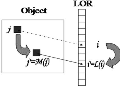
Fig. 1. An event detected at an LOR  $i'$  generated in voxel  $j$ , which has been translated to voxel  $j' = \mathcal{M}(j)$  at time of detection, would have been detected at LOR  $i = \mathcal{L}^{-1}(i')$  if the object had not moved.
