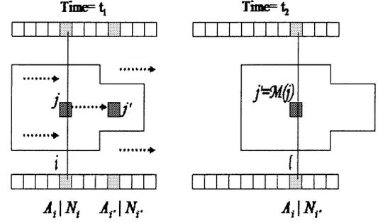
Fig. 2. Event detected at time  $t_2$  along an LOR  $i'$ , which would have been detected along an LOR  $i$  if the object had not moved, has the *same* attenuation correction factor as measured for  $A_i$  at time  $t_1$ . The normalization correction factor, however, is LOR-specific and changes with motion.
