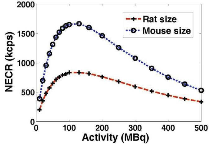
Fig. 3. Plots of simulated NECR as a function of total activity for mouse- and rat-sized phantoms.
