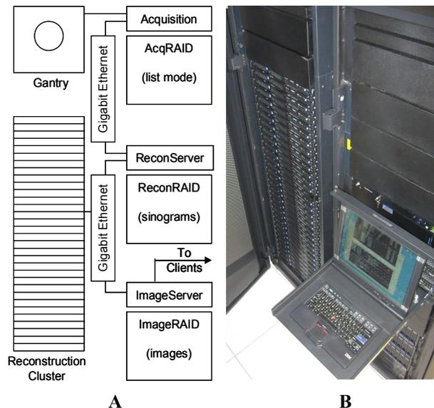
Fig. 3 (A) General computer architecture of the HRRT data processing system. (B) Photograph of the installed system. The 32-node (64 processor) reconstruction cluster is contained in the left rack; the ReconServer, the ImageServer, and the mass storage RAID's are contained in the right rack. The acquisition computer is not illustrated.
