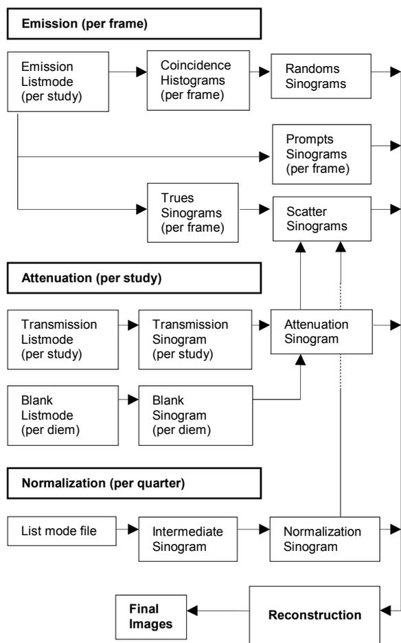
Fig. 2 Data processing chart for HRRT image reconstruction.
