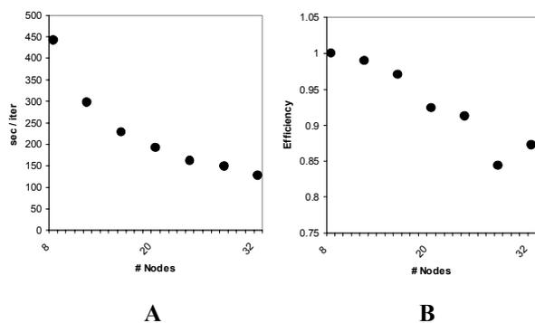
Fig. 4 (A) Ordinary Poisson OSEM3D reconstruction time per iteration for HRRT span-3 data as a function of the number of nodes in a cluster. Speedup is obtained through 32 nodes. (B) Efficiency of the calculation relative to the 8-node case. High efficiency can be retained by reconstructing multiple frames in parallel using *multicluster* methods.
