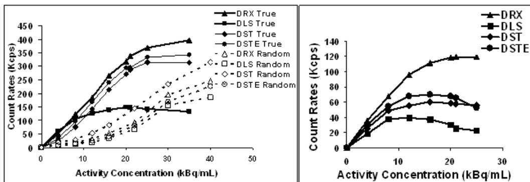
**Figure 6.** Random and True rates vs. activity concentration (left). NECR vs. activity concentration for GE PET cameras (right). The object imaged was the NEMA 2001 scatter phantom. The random event rates were divided by a factor of 5 to enable both rates shown in one figure.
